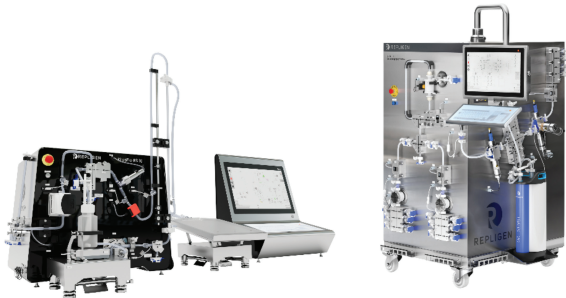
Figure 3. KrosFlo® RS TFF Systems (left) and KRM™ Chromatography Systems from Repligen minimize users' exposure to hazardous materials during manufacturing processes.
