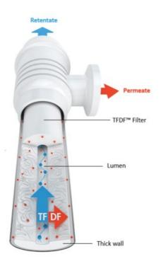
Figure 2. Tangential flow depth filtration (TFDF<sup>®</sup>) operates a depth filter in tangential mode. Cell culture medium passes through the lumen of the tubular depth filter. Permeate passes through the depth filter wall and exits a permeate port. Retentate exits the lumen and directed back to the bioreactor.
