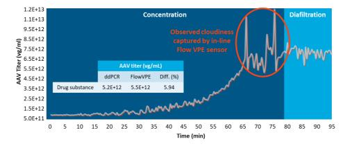
Figure 5. In-line measurement of AAV titer during final concentration and diafiltration process steps using the Slope Spectroscopy® FlowVPE® technique. In-line monitoring enables rapid adjustment as process deviation occurs (e.g. cloudiness observed, indicating potential virus aggregation, requires stopping concentration and/or changing buffer).
