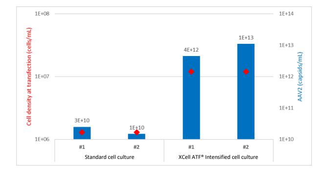
Figure 1. Intensification of AAV2 production process with XCell ATF<sup>®</sup> (data adapted from (14), courtesy of Cytovance<sup>®</sup> Biologics). The AAV2 productivity of a perfusion process using the XCell ATF<sup>®</sup> cell intensification device (immediately prior to` transfection) increased capsid production > 100-fold relative to the standard batch process.
