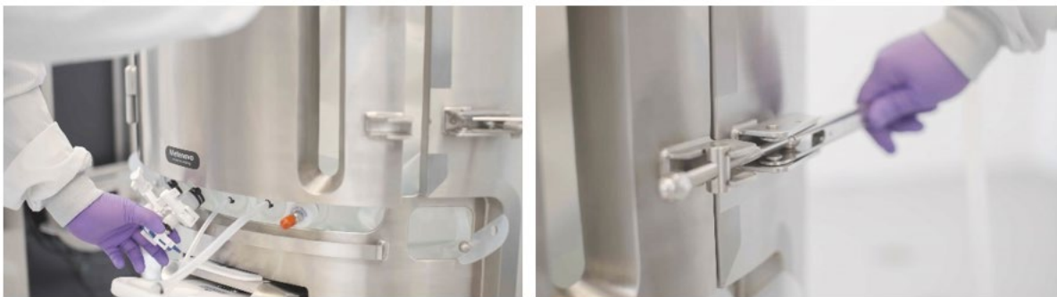
Figure 64. Installing the security pin
