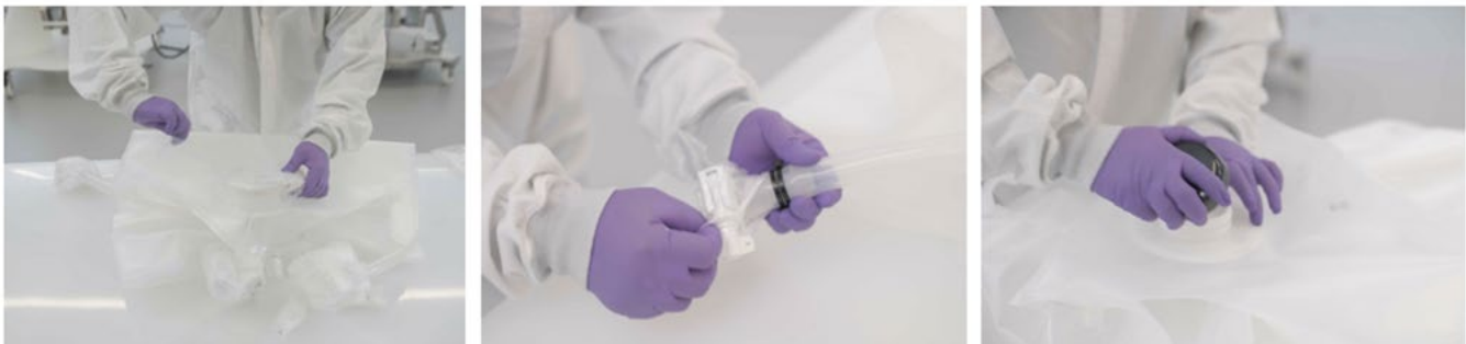
Figure 46. Removing the Bubble Wrap and Vinyl Tank Plate Cover
