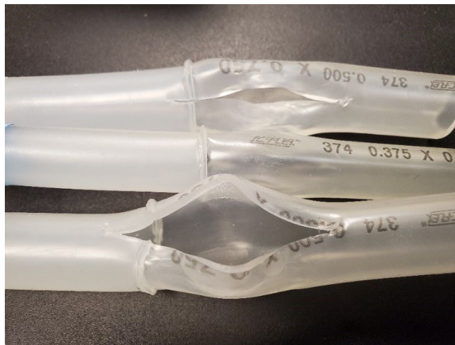
Figure 3. Burst tubing example
