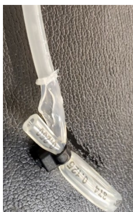
Figure 4. Burst away from weld example
