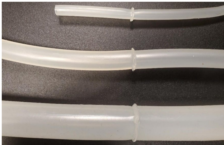
Figure 1. Tube weld example
