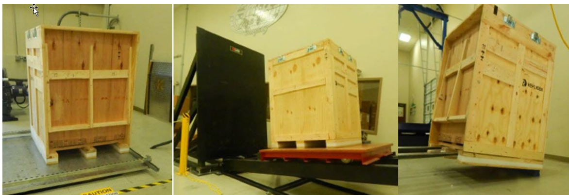
Figure 30. OPUS 60R Pre-packed Chromatography Column Vibrational, Incline Impact, Drop Testing
