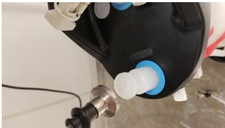
**Figure 19. Connect rigid tubing to small column outlet and inlet**
