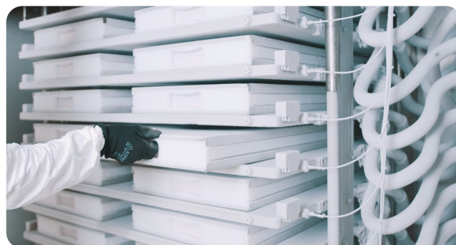
Figure 4: Frozen RoSS® shells in a plate-based freezing system
