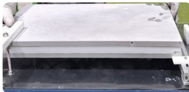
Figure 5: Low-temperature performance testing of the RoSS® shell with ProConnex® 2D bag assembly
