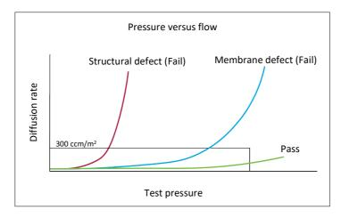
Air Integrity testing for ultrafiltration cassettes can identify both membrane defects as well as structural cassette defects at  $300 \text{ ccm/m}^2$  and 1 bar (14.5 psi).
