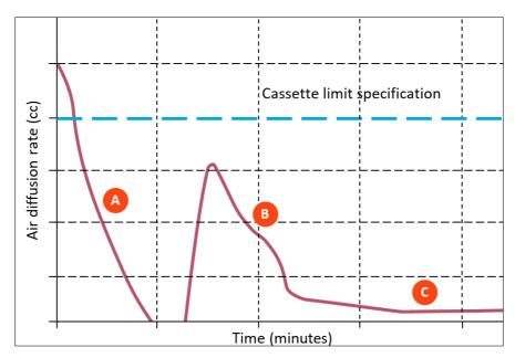
Figure 9. Integrity test air diffusion rate
