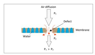
When a defect is present in the TFF cassette, air will easily pass through the opening. The increased air flow is easily detected and indicates a defect is present.
