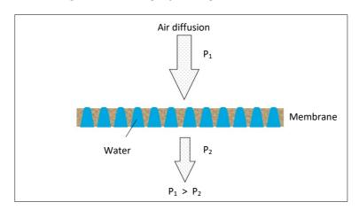
Figure 2. Air Integrity testing for TFF cassette
