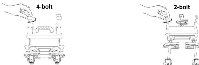
2. Using the calibrated torque wrench tighten each hex nut 1/4 turn at a time following the torque sequence illustrated in (4-bolt pictured above) or (2-bolt pictured above).
