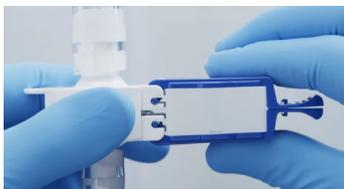
4. Pull on the two blue interlocked tabs to remove the membrane from the connectors.
