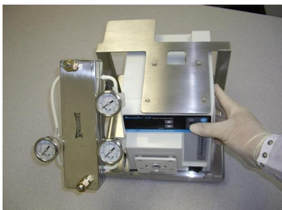
5. Mount pump head onto the pump. See the Easy-Load® 3 pump head operating manual for instructions.
