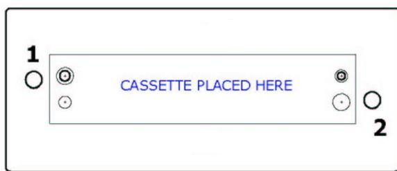
**CAUTION: NUTS MUST BE TIGHTENED UNIFORMLY TO AVOID DAMAGING THE CASSETTE. LEAKAGE MAY RESULT FROM NON-PARALLEL PLATE ALIGNMENT OR OVER COMPRESSION OF THE CASSETTES AT ONE END.**
