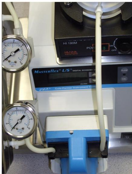
6. Connection is made by gently pushing the tubing onto the barbed fitting and turning the tubing cap clockwise until the tubing is secure.
