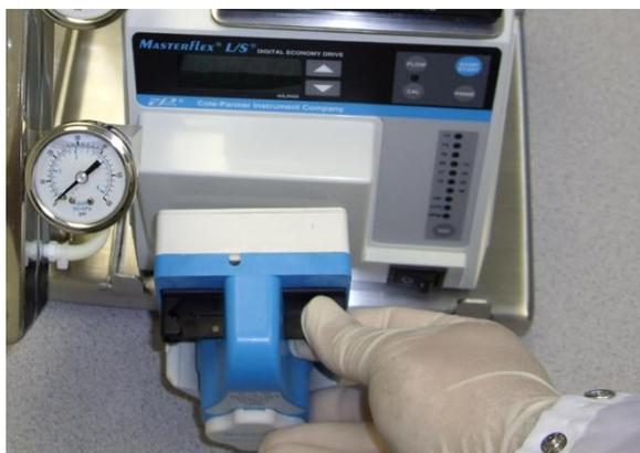
6. Pump head should be mounted so that the tubing will enter and exit vertically in the upwards position when loaded.
