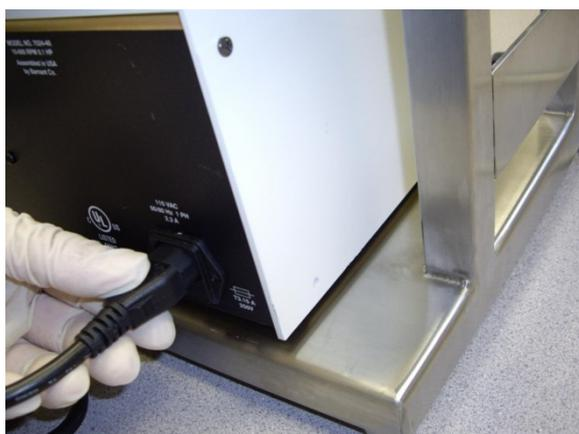
8. Ensure the plug is not tangled at the back of the pump and is within easy reach of an electrical outlet.
