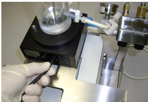
4. Ensure the plug is not tangled at the back of the magnetic stirrer and is within easy reach of an electrical outlet.
