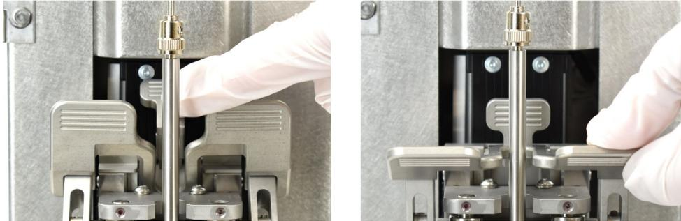
Figure 7. Closing Fibrette Clamp over Flow Fibrette.
