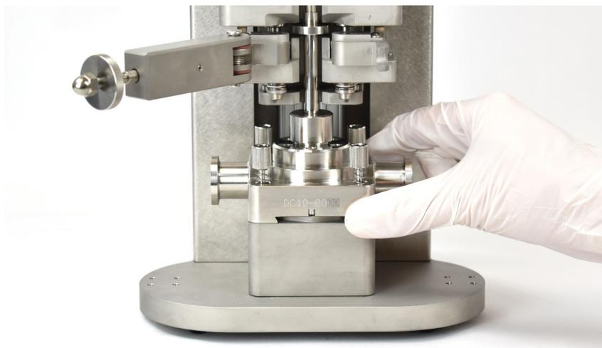
Figure 5. Flow Cell mounting to Flow Head.
