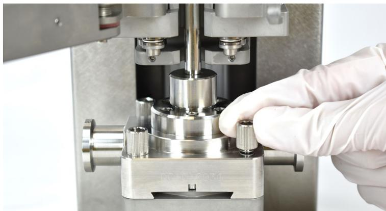
Figure 6. Securing Flow Cell to Detector Module.
