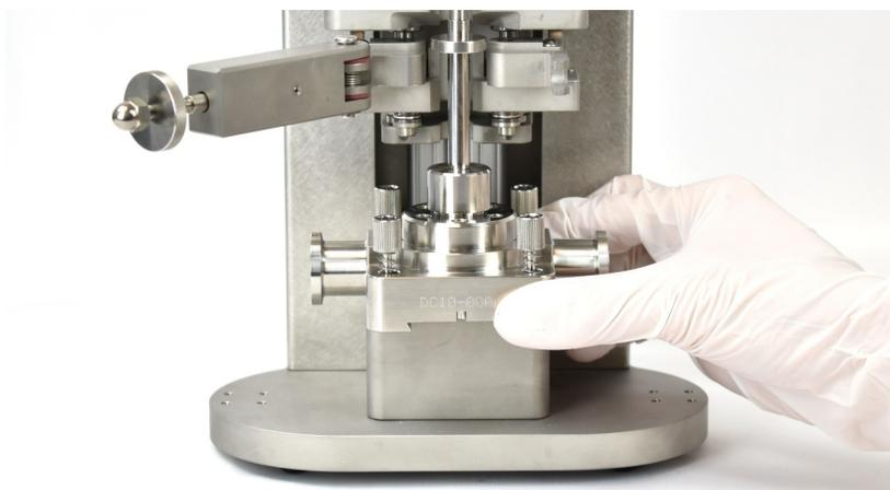
Figure 4. Flow Fibrette Flange fitting into Fibrette clamp.
