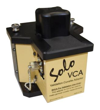
The SVCA is simple to install and run using the Cary WinUV Validation program available on the system. With the SoloVPE Validation Cuvette Adapter (SVCA), traditional UV-Vis spectrophotometric filter standards can be run on the SoloVPE sample detector. NIST traceable filter standards such as neutral density or sealed liquid standards are compatible. Metal on quartz filters not currently compatible.
