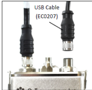
Figure 33. USB Cable (EC0207) to FlowVPX Head
