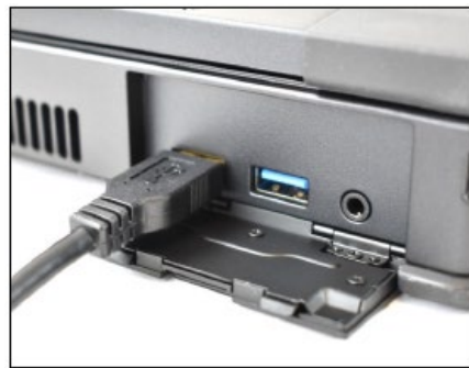
Figure 34. FlowVPX USB cable (EC0207) to computer
