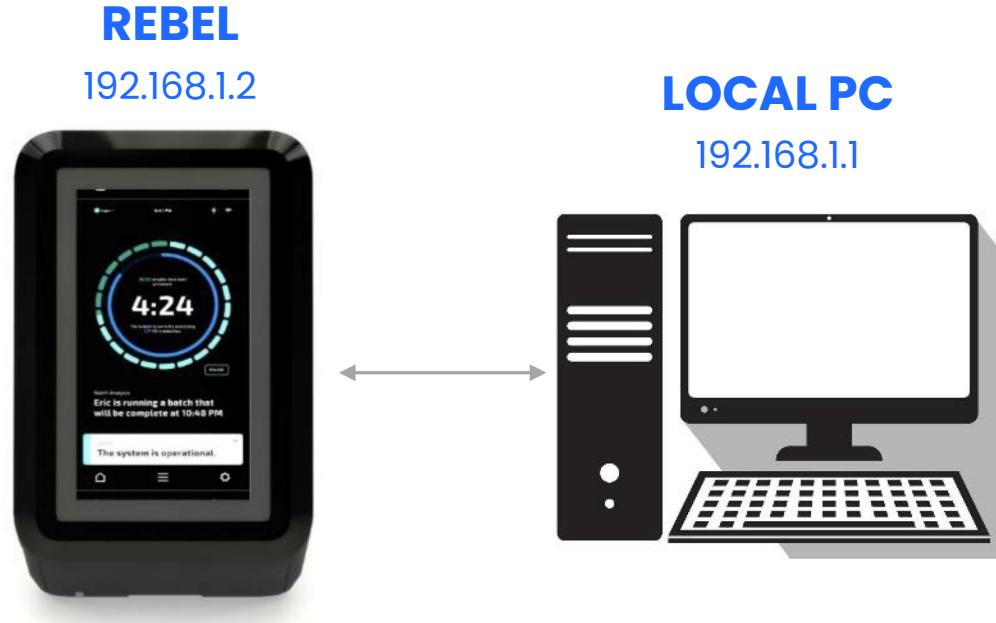
Connect through local hub or directly with ethernet cable.
