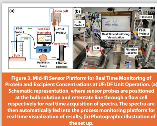
**Figure 3. Mid-IR Sensor Platform for Real Time Monitoring of Protein and Excipient Concentrations at UF/DF Unit Operation. (a) Schematic representation, where sensor probes are positioned at the bulk solution and retentate line through a flow cell respectively for real time acquisition of spectra. The spectra are then automatically fed into the process monitoring platform for real time visualization of results; (b) Photographic illustration of the set up.**
