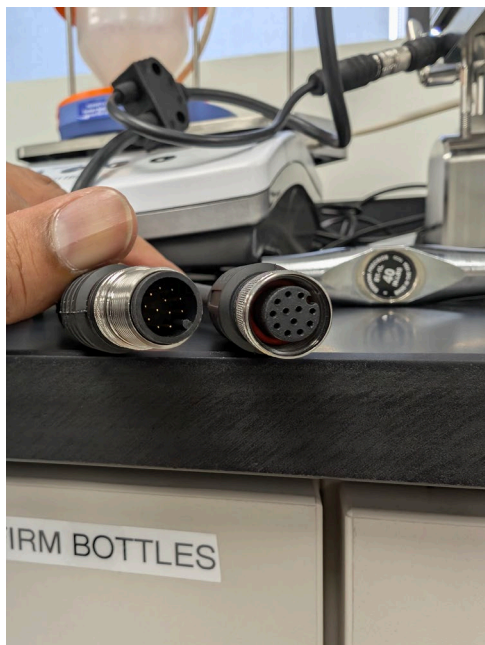
Figure 13. RSKV-12 cable connection with splitter cable.
