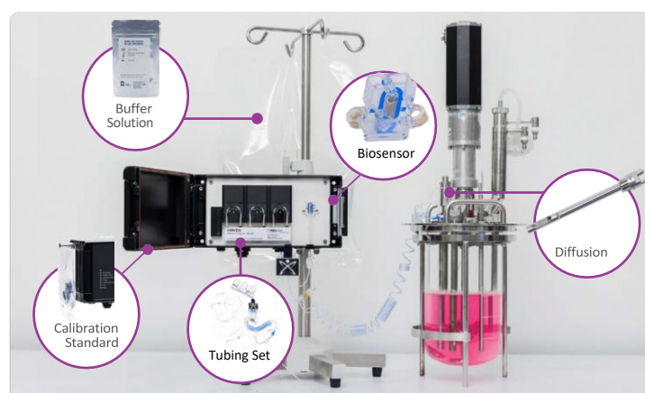
Figure 1. MAVEN System components and connection to a 2 L, single-walled bioreactor from Sartorius
