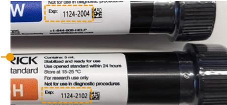
**Note:** Location of serial numbers on calibration standard vials. Entering expired or incorrect codes will result in an error message.
