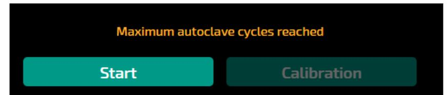
**Note:** If the maximum number of autoclave cycles have been reached, the system will still allow you to start a Session but will use the last stored probe calibration data. This functionality should only be used in exceptional cases where a session was stopped inadvertently after the final autoclave cycle.
