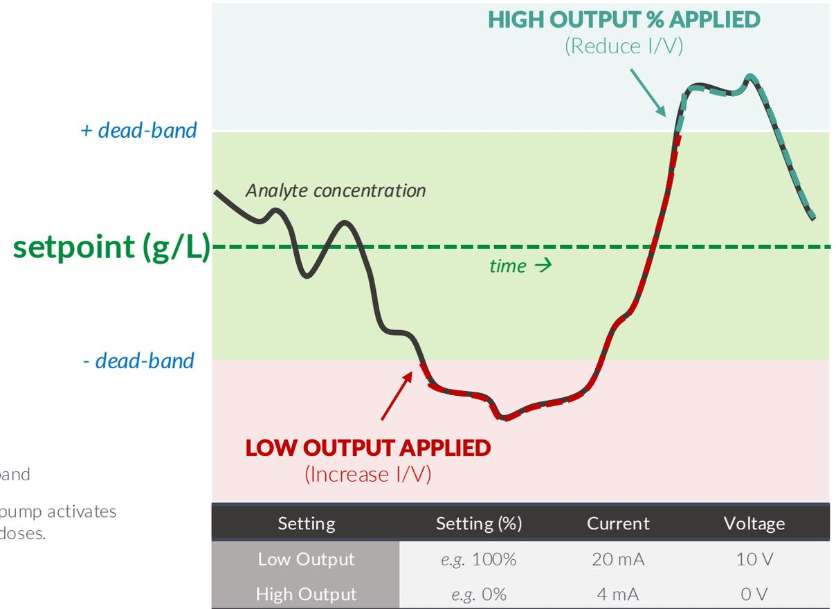
An illustration of MAVERICK as a pump controller, with example values below. When concentration declines below the lower deadband, the low output feed setting is applied until concentration reaches above upper deadband, whereupon the high output feed setting is applied.
