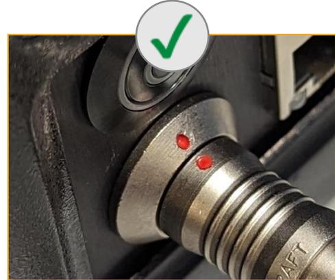
**Caution:** Ensure the power plug is firmly seated into the back of the Hub without gaps.
