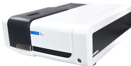
The SoloVPE instrument functions by drawing its power directly from the Agilent Technologies Cary 60 UV-Vis spectrophotometer. The Cary 60 requires a Dual Use Fiber Optic Coupler, provided by Repligen's Analytics business unit, to ensure adequate light transmission through the Fiber Optic Cable to the SoloVPE instrument.
