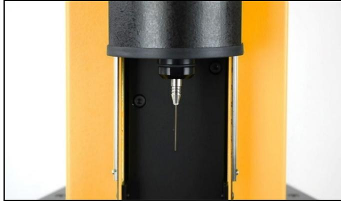
Figure 9. Quick Set Coupler with Fibrette Optical Component inserted.
