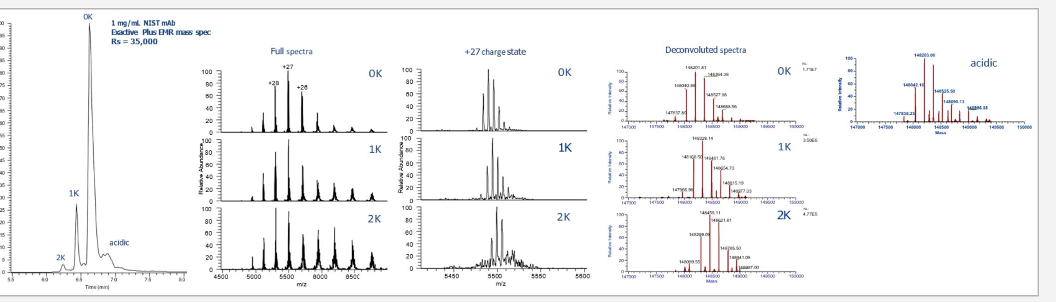
Microchip CE-MS separation of the NIST mAb under native conditions yields baseline resolution of the C-terminal lysine variants (2K, 1K and 0K), and resolution of one or more acidic variants. Resolution of these variants in the front end separation greatly improves the mass spec's ability to clearly identify the variants. The acidic variants have very small mass shifts, likely attributable to deamidations.
