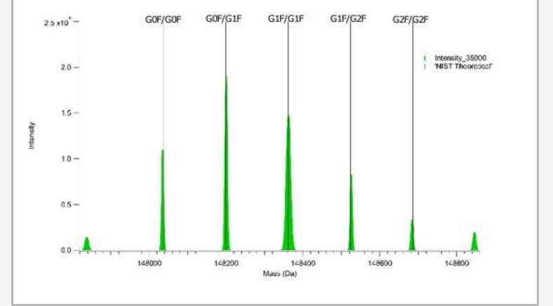
As others have previously shown, the orbitrap can achieve high resolution and mass accuracy of large intact proteins, but the signal intensity decays at higher resolution settings. We observed high mass accuracy at all resolution settings, with optimal glycoform resolution at a setting of 35,000. The plot above shows the deconvoluted spectrum acquired at 35,000 resolution compared to the theoretical masses. The measured mass error was 0.7 Da (~5 ppm).
