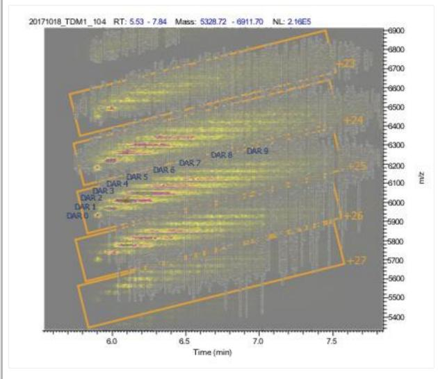
Conjugation of drug molecules onto the structure of trastuzumab creates a very complex group of variants. Without a separation, spectral overlap impedes the mass spec's ability to see all of the drugantibody ratio (DAR) variant peaks. The 2D map view shows how the combined power of the separation and the mass spec can resolve all of the variants.
