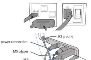
**3** Connect cables between ZCI, MS and control computer.
