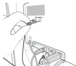
**4** Connect BGE and sample transfer lines from AS to ZCI (if equipped).
