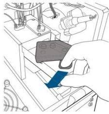
**3** Place a ZipChip in the tray. Pull back the chip latch to seat it in the chip tray.
