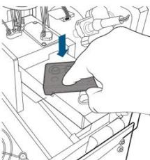
**4** Lightly press down on the chip to secure it in the tray.
