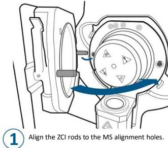
**1** Align the ZCI rods to the MS alignment holes.
