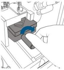
**1** Rotate the chip loading lever.
