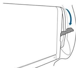
**2** Rotate locking levers down to engage.
