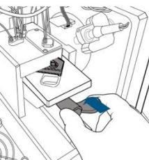
**5** Slide the chip tray back into the chip manifold.
