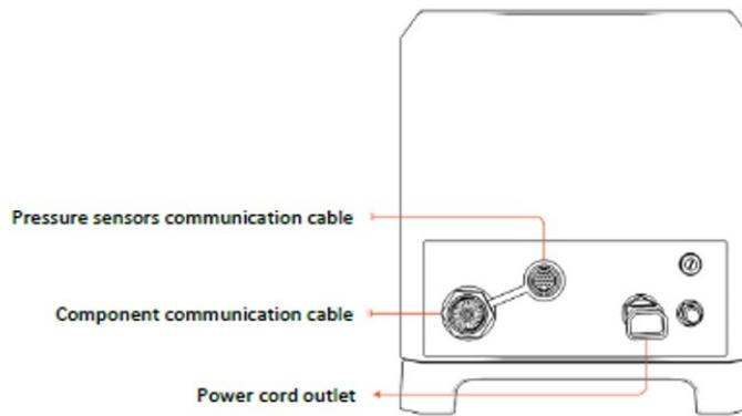
Figure 31. KR2i Auxiliary Component Cable
