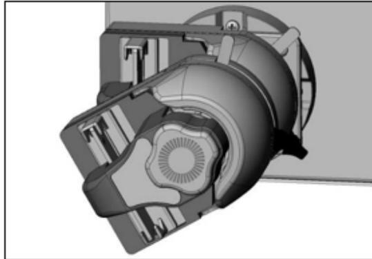
Figure 14. Drive With Both Pump Heads Locked in Position
