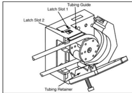
Figure 19. Closing Occlusion Bed of Easy-Load Pump Head
