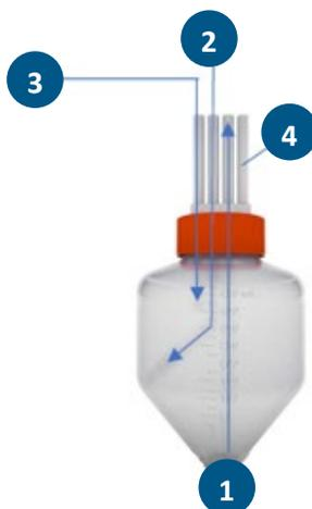
Alternatively, an additional feed vessel may be set up to draw a vacuum. To create a vacuum, on the primary feed reservoir, set up four ports (Figure 3) to draw excess feed into the primary reservoir from the additional feed vessel:
