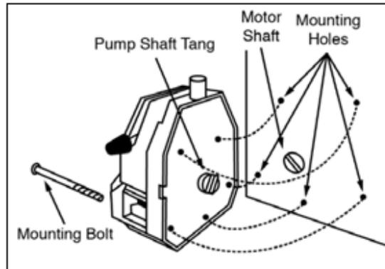
Figure 16. Components of the High-Performance Pump Head
