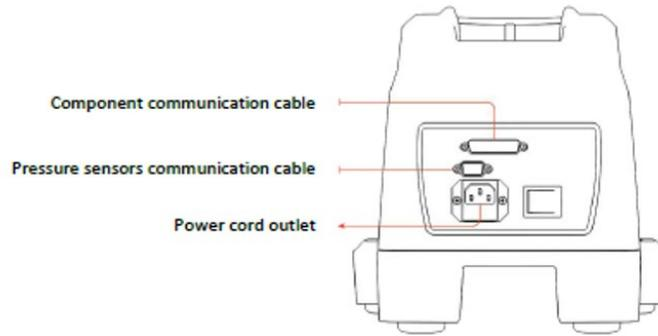
Figure 30. KrosFlo KMPi TFF System Cable Connections
