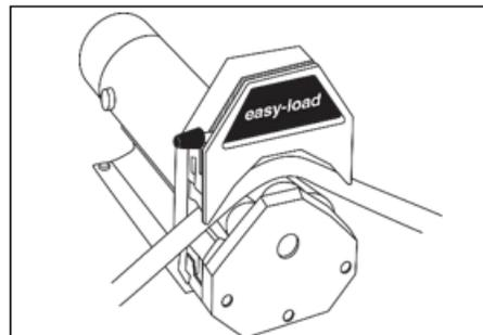
Figure 18. Loading Tubing into Open Occlusion Bed of High-Performance Pump Head
