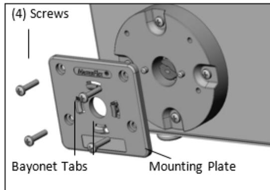
Figure 6. Back of Research II Pump Head
