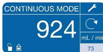
If pump shows "----" after starting up (Figure 27), it is in remote control mode and is ready to use. If pump shows a flowrate after starting (Figure 28), it needs to be set to remote control mode.
