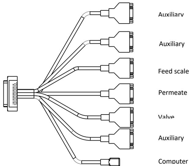
Figure 32. KMPi Auxiliary Component Cable
