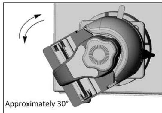
Figure 8. Bayonet Feature Locked in Horizontal Pump Orientation
