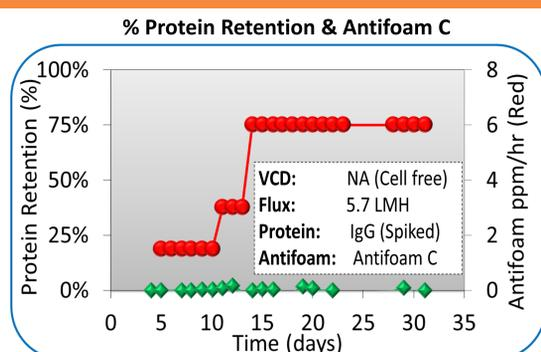
Data from above experiment (spiking antifoam-C and IgG to a cell free perfusion system) indicated that Antifoam-C has no impact on protein retention.
