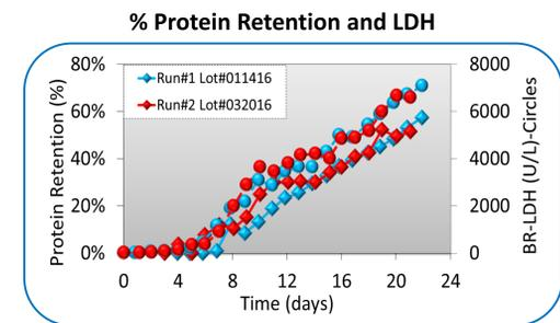
Protein retention and LDH profiles correlated well in both test runs, indicating that cell lysis (cell debris) plays a crucial role in protein retention
