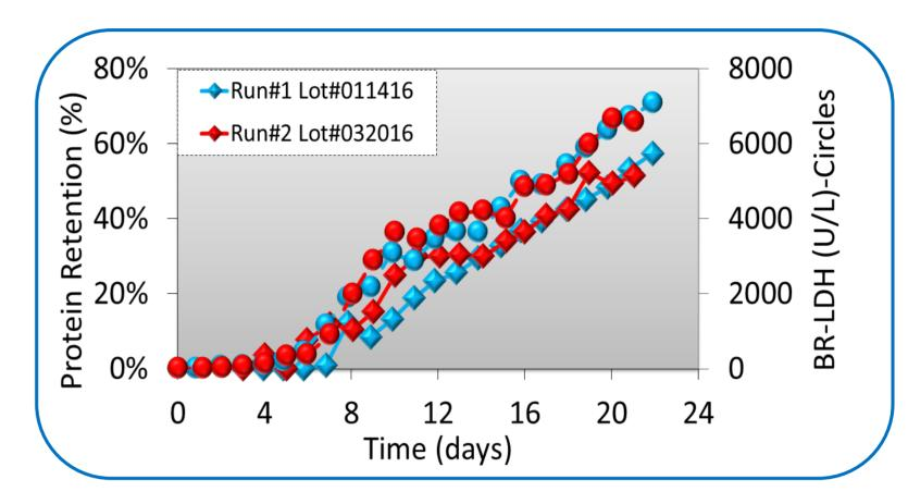
Protein retention and LDH profiles correlated well in both test runs, indicating that cell lysis (cell debris) plays a crucial role in protein retention
