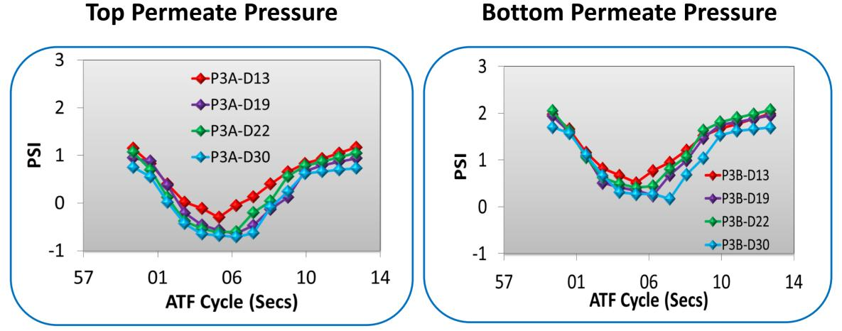
Based on the above experiment, antifoam C alone has no impact on protein retention (based on protein conc.) and filter fouling (based on permeate pressure)
