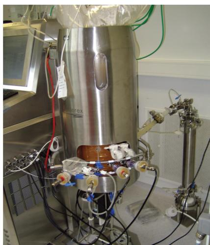
An Xcellerex bioreactor used in an intensified perfusion process with ATF System equipment ([WWW.REFINETECH.COM](http://WWW.REFINETECH.COM))
