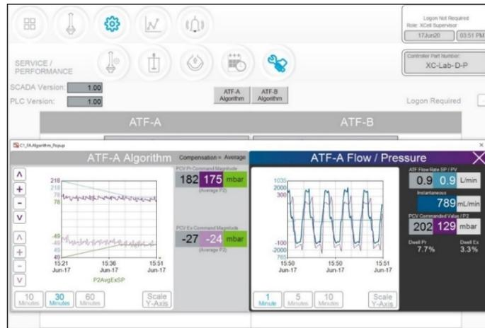
Clicking the **Algorithm** button displays a pop-up (Figures 28, 29), which shows various flow/pressure signals while the controller is running. This screen displays various signals and messages. It is not advisable to judge the algorithm performance without significant training and experience since the data can be misinterpreted. This screen is used by Repligen FAS during troubleshooting. Please consult a Repligen FAS if you suspect your XCell ATF Devices are not working satisfactorily.
