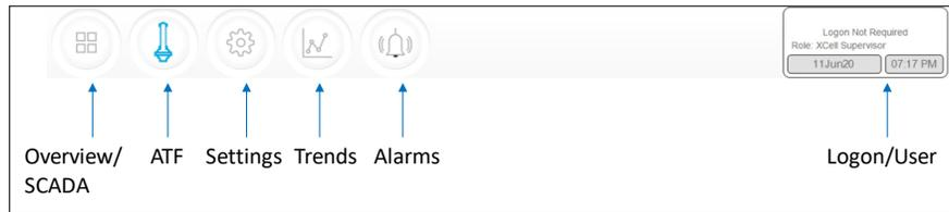
The menu bar displays six options at the top of the screen (Figure 11). The blue highlighted button indicates the screen currently active. To change to another screen, just press one of the other buttons.
