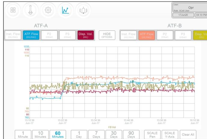
The XCell Lab Trend screen displays flows, pressures and displacement volumes for each XCell ATF Device ([Figure 30](#)). By clicking on the various buttons, you can select and simultaneously display multiple parameters. The buttons are colored if selected and greyed if not. Graph line colors are predetermined and cannot be modified.
