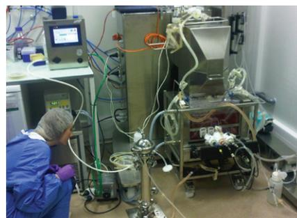
**Microcarrier-based perfusion in a single-use ATMI bioreactor** ([WWW.REFINETECH.COM](http://WWW.REFINETECH.COM))
