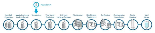
Figure 1. AAV production process containing two TFF steps
