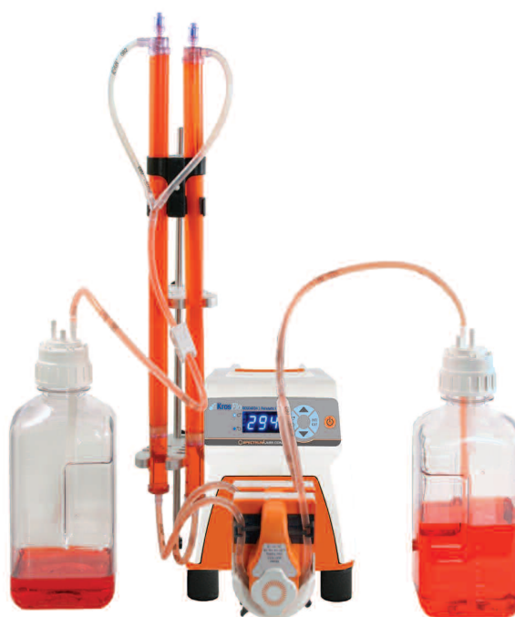
Coupled Tube-A-Lyzer® units set-up for parallel operation in single-pass mode
