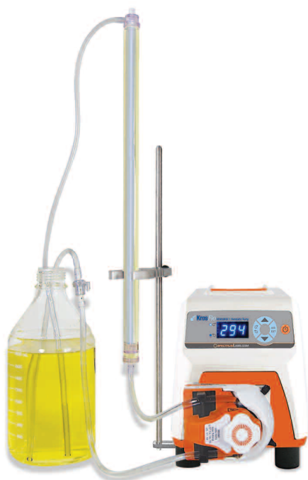
Single Tube-A-Lyzer® unit set-up on KrosFlo® Research III Pump for buffer re-circulation
