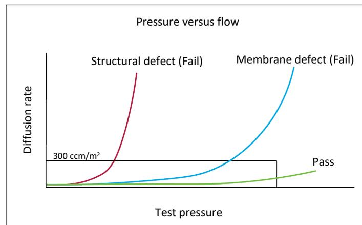
Air Integrity testing for ultrafiltration cassettes can identify both membrane defects as well as structural cassette defects at 300 ccm/m<sup>2</sup> and 1 bar (14.5 psi).
