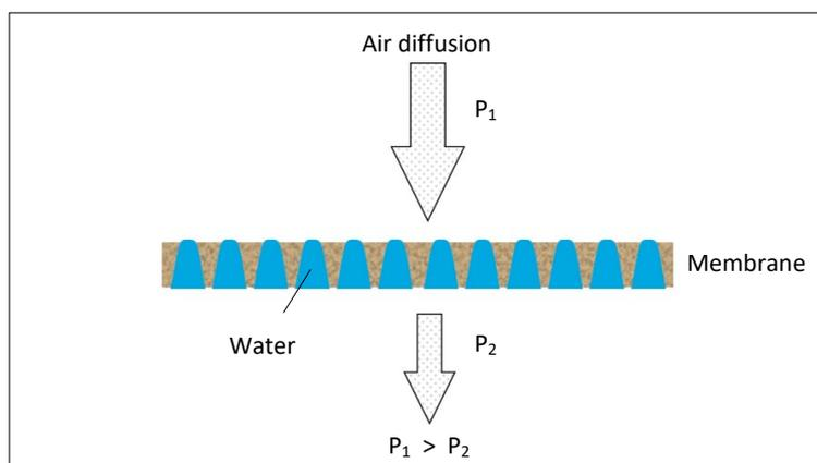
Air Integrity is measured at a pressure below the membrane's bubble point. Only minimal amount of air diffusing through the liquid will pass from the feed to permeate.
