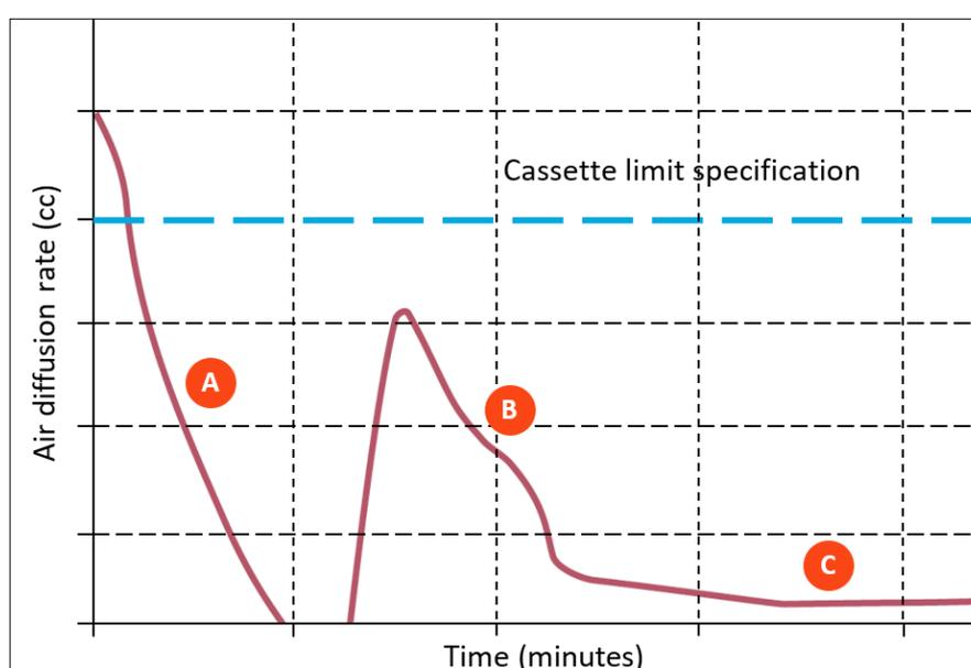
**Example:** Typical air (mass) flow rate plotted for an integrity check of a system and membrane cassettes: A = System test B = Membrane test C = Diffusion rate.
