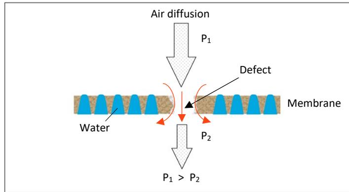
When a defect is present in the TFF cassette, air will easily pass through the opening. The increased air flow is easily detected and indicates a defect is present.
