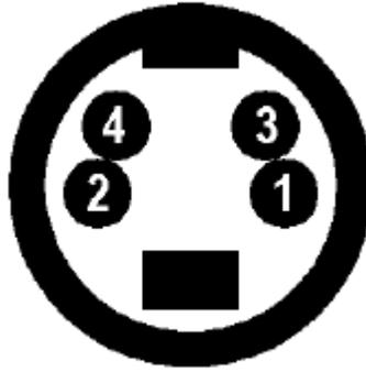
Figure 4-2. Event Connector on Rear Panel.
