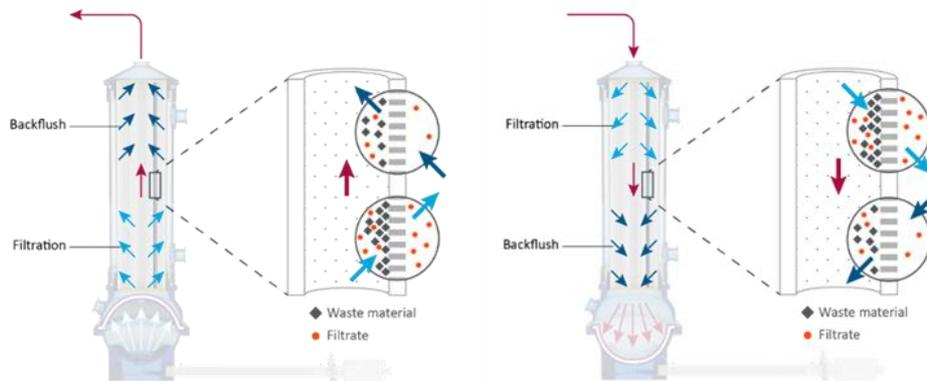
**Figure 1.** XCell ATF® Technology extends filter lifetime by utilizing a diaphragm pump to provide alternating tangential flow through a hollow fiber filter, back and forth between the device and the bioreactor.
