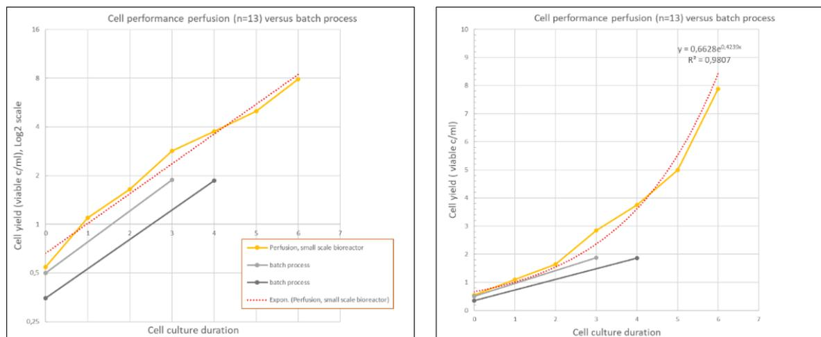
**Figure 2a and 2b.** Cell growth curve showing viable cell yield as Log2 scale (2a, left) and linear scale (2b, right) versus cell culture duration (x-axis, days post cell seeding) of the reference batch processes (culture without medium refreshment) versus perfused cells. The dotted line represents the exponential trend line of the perfused cultures.
