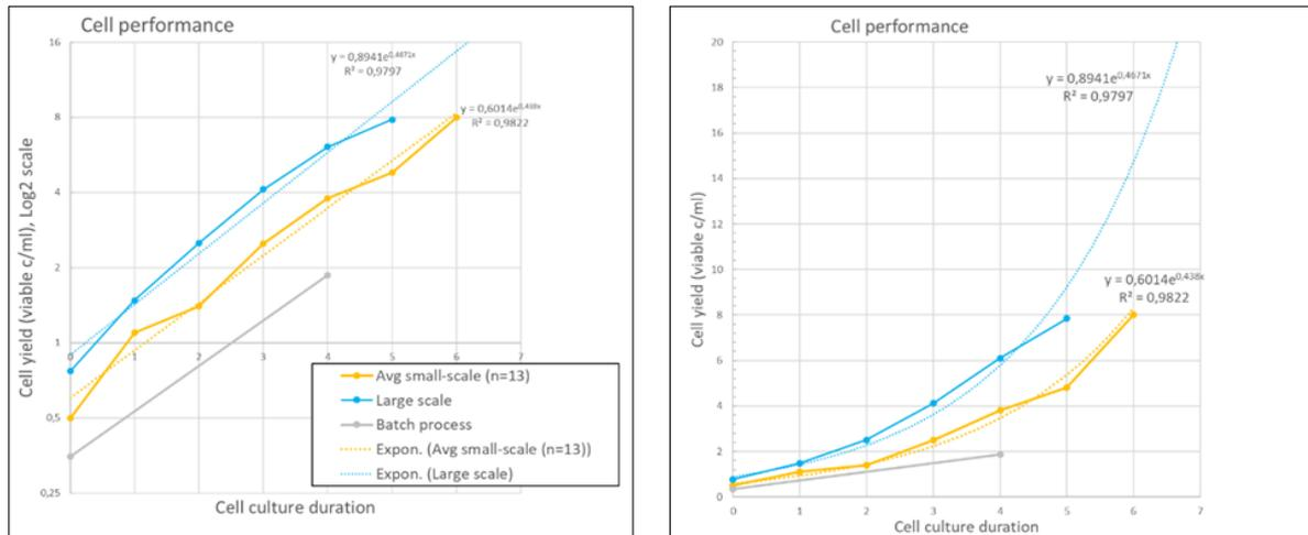
**Figure 5a and 5b.** Cell growth curve showing viable cell yield as Log2 scale (5a, left) and as linear scale (5b, right). The blue curve represents the large-scale perfusion batch, the yellow curve the average of small-scale cultures (n=13). The dotted lines represent the exponential trend lines of the perfused cultures. Reference batch process is plotted in grey.
