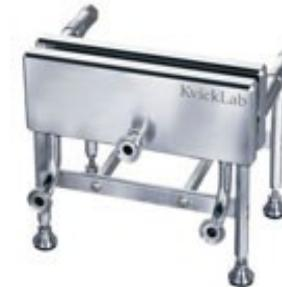
The TangenX™ PRO cassette must be placed in the cassette holder with the identification label facing away from the feed/retentate ports and towards the brass retaining nuts. The recommended torque values are shown below.
