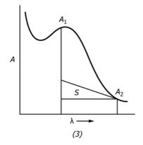
where the subscripts refer to analytical wavelengths. The term  $A_2$  is the absorbance at the wavelength used for making a simple subtractive correction. It is usually selected from examination of the spectral curve of the reference material at a wavelength longer than that of  $A_1$ , preferably where  $a_2$  is much less than  $a_1$ .
