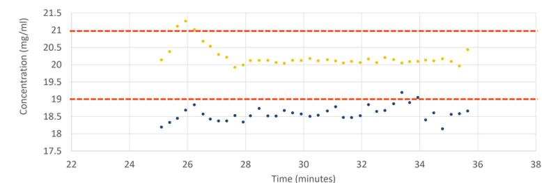
Figure 8. Low concentration diafiltration compared to desired concentration.
