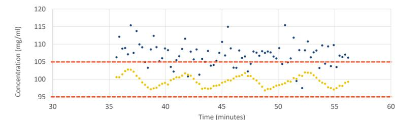
Figure 9. High concentration diafiltration compared to desired concentration.
