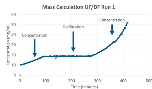
Figure 4. Mass calculation of UF/DF run 1.
