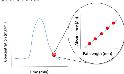
Figure 1. Beer-Lambert law and the Slope Spectroscopy equation.
