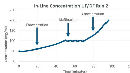
Figure 7. In-line concentration of UF/DF run 2.
