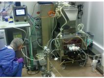
Microcarrier-based perfusion in a single-use ATMI bioreactor (WWW.REFINETECH.COM)
