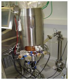
An Xcellerex bioreactor used in an intensified perfusion process with ATF System equipment (WWW.REFINETECH.COM)
